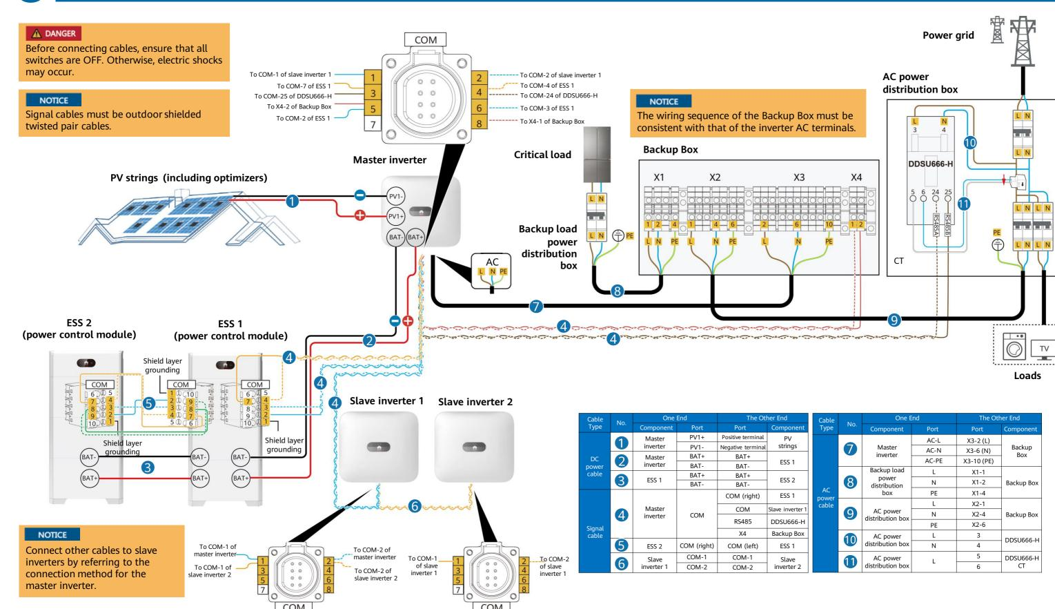
(Single-Phase PV+ESS Scenario + Smart Dongle Networking)
