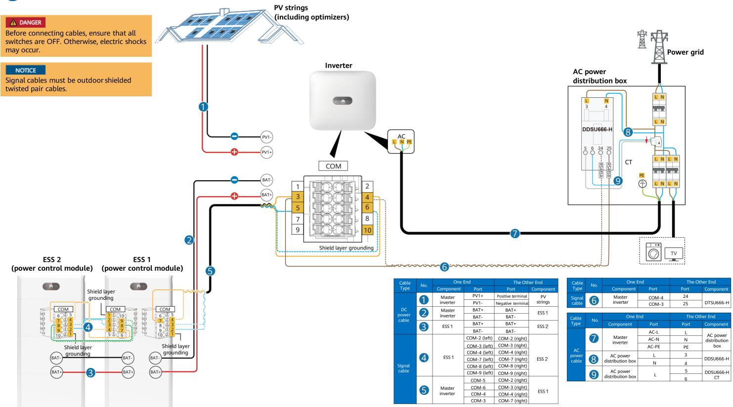
(Single-Phase PV+ESS Scenario + Smart Dongle Networking)
